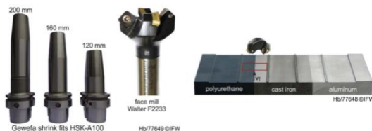
Fig.8 Milling of Polyurethane, Cast Iron, Aluminium materials by varying length shrink fit holders
